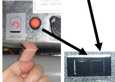
Location of switch on an electric fryer is behind the far right control box.
